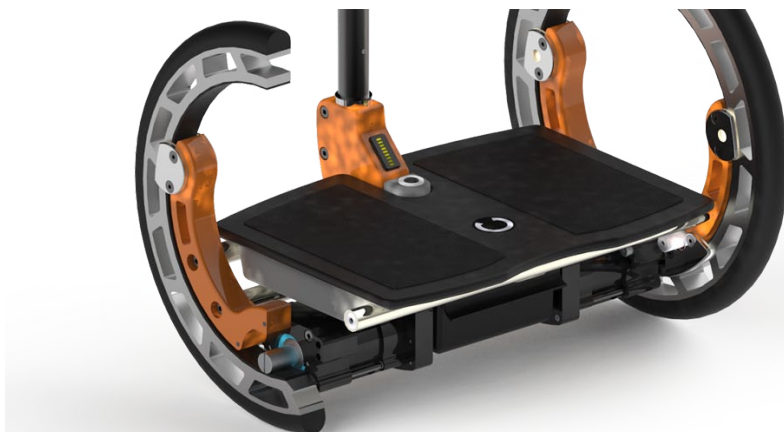
The motors' axles directly sit on the internal rim of the hub-less wheels.
