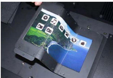
Triptych 5.9-inch AMOLED display. Source: Japanese research institute Semiconductor Energy
