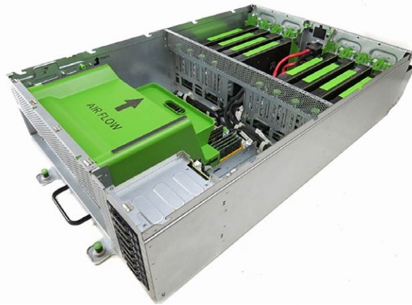
Big Sur packs eight Nvidia Tesla M40 accelerators using an OpenCL interface, but is qualified to handle other PCI Express cards. (Image: Facebook)
